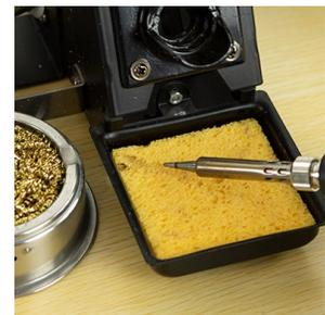
Repeat if necessary until visibly clean and remember you don't want to be poking the sponge with the tip of the iron, the whole surface should be making contact.
