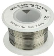
The easiest method of applying flux is through flux-cored solder wire. As the name implies, there is one or more cores of flux present throughout the length of the solder wire. It is formulated so that when you melt the solder, the perfect pre-measured amount of flux is also applied. The percentage of flux to wire is typically between 1-3% and will usually be printed on the label. The higher the flux content, the more active it will be in removing oxides.
