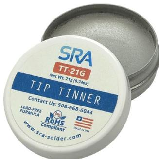
Tip Tinner is a compressed tablet that contains a mixture of solder and oxide reducing compounds. Used for safe cleaning and re-tinning of oxidized soldering iron tips. It is preferred over solder wire because it does not contain any harmful flux acids that can reduce the life of your tip and is less wasteful. Tinning is discussed in-depth at rule #9.
