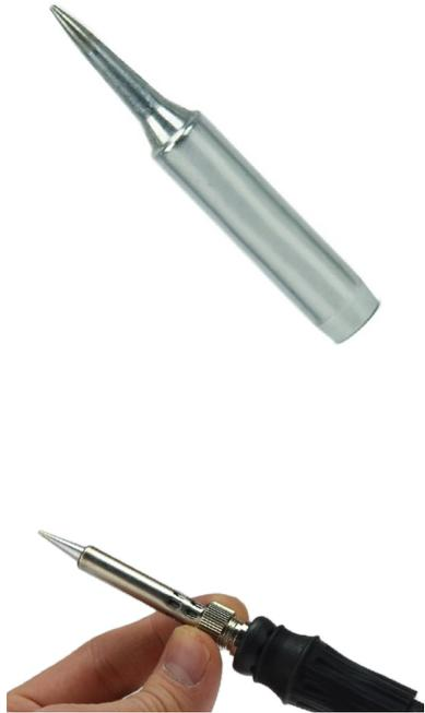
These standard tips are most commonly found on modern irons. They are partially hollow and slide onto the heating element of the iron. In order to replace them, the metal shield that protects the element must be removed first. These tips are great because they last a long time and are sometimes compatible across brands. Some models will use a set screw to keep the tip in place instead but they are often lower quality.
