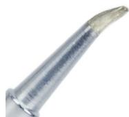
**RB Tips** - These tips have a small bend of about 30° very close to the end of the tip. It is used for drag soldering and the fixing of solder bridges.
