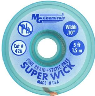
A desoldering wick is simply a roll of copper mesh that is infused with flux. Usually it is either a rosin or no-clean type flux and when heated it draws the solder out of the joint. The solder wick is best used on SMD components and joints with little solder to remove.
