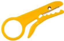
A step up from the hobby knife but similar idea. The jaw holds the wire in the appropriate groove and allows you to score around the insulation using your finger through the loop. These work great for larger shielded cables.
