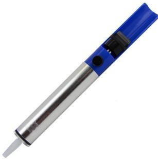
If you've got a lot of solder to remove, the desoldering pump or "solder sucker" is a must. When the plunger is engaged, a vacuum is created. The heat resistant teflon tip can then be placed at the joint and when the button is pressed, it sucks the molten solder right out. The design is semi self-cleaning but they do get jammed and must be cleaned out before continuing.
